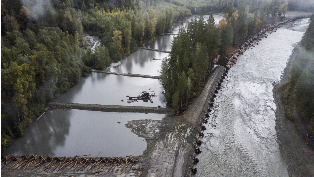
The South Fork Stillaguamish River runs through a new location past a man-made meander jam, a large woody material jam, and a live crib wall to help guide its new course in Verlot. (Olivia Vanni / The Herald)
